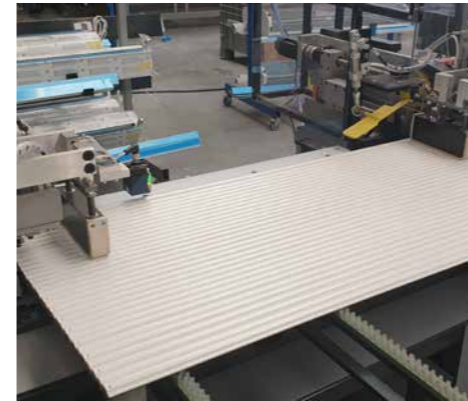
Machine for cutting and assembling aluminium roller shutter apron
