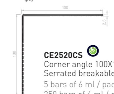
**CE2520CS** Corner angle 100X100X2,5-2 Serrated breakable
