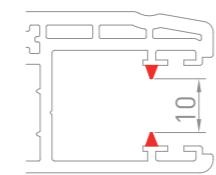
NB : the bioclimatic slat is used with the PVC guide and the coextruded joint : **JC10**
