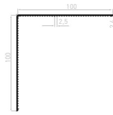
**CE2420C** Angle section 100X100X2,4 Serrated
