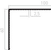
**CE2421C** Angle section 100X60X2,4 Serrated
