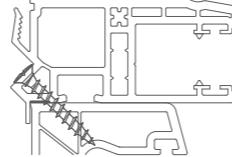
The **blocks** are all to be fixed with an SFS reference stud screw : SPK/5-74/GS - 4x10
