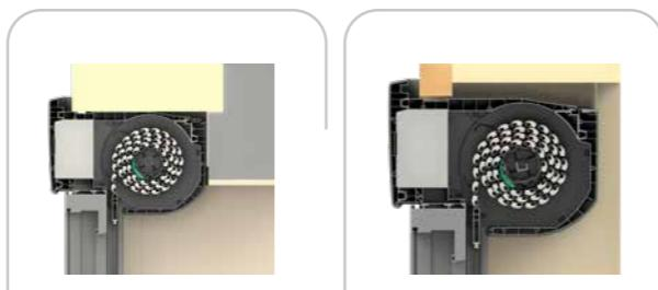
Installation as external thermal insulation
