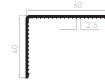
**CE2430C** Angle section 60x40x2,4 Serrated
