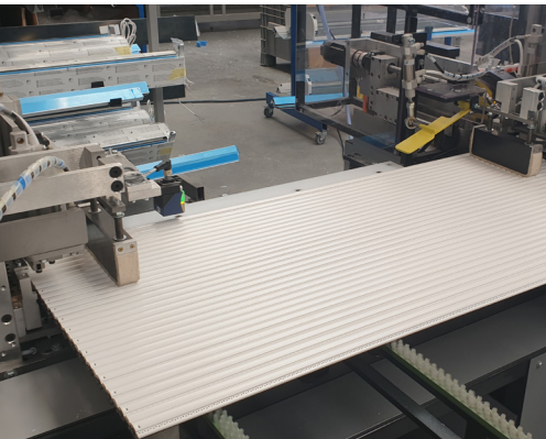
Machine for cutting and assembling aluminium roller shutter apron
