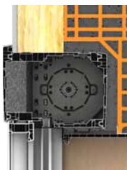
Half-lintel installation (1 st floor access through interior hatch)
