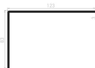
CE3015 Corner angle 123X83X3 5 bars of 6 ml / pack 200 bars of 6 ml / container
