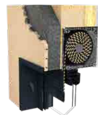
Installation on timber- frame house
