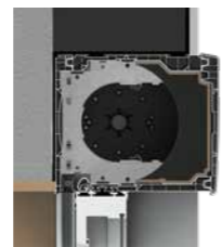
Installation as external thermal insulation
