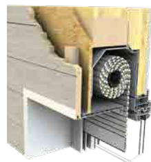
Installation on timber-frame house
