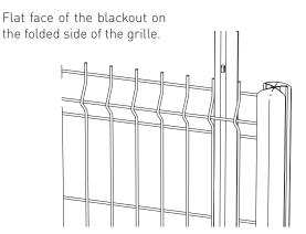
Lower the blackout until the clip locks into the mesh wire.
