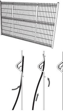
Once the angles are in position, insert the top of the blinds between the locking angle and the horizontal wires, bending them until they lock into place.
