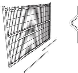
Position the reinforcing angles in the bottom and middle folds of the grille. Hold them in place by slipping a blackout slat between each length of angle and the horizontal wires.
