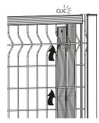
Leave the meshes at the ends of the grid empty, then braid with the widest plates, starting from the bottom and working your way up. Repeat the process until you have filled the grid.
