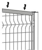
Place the finishing clip at the top of the panel with the flat side facing the folds of the grille.
